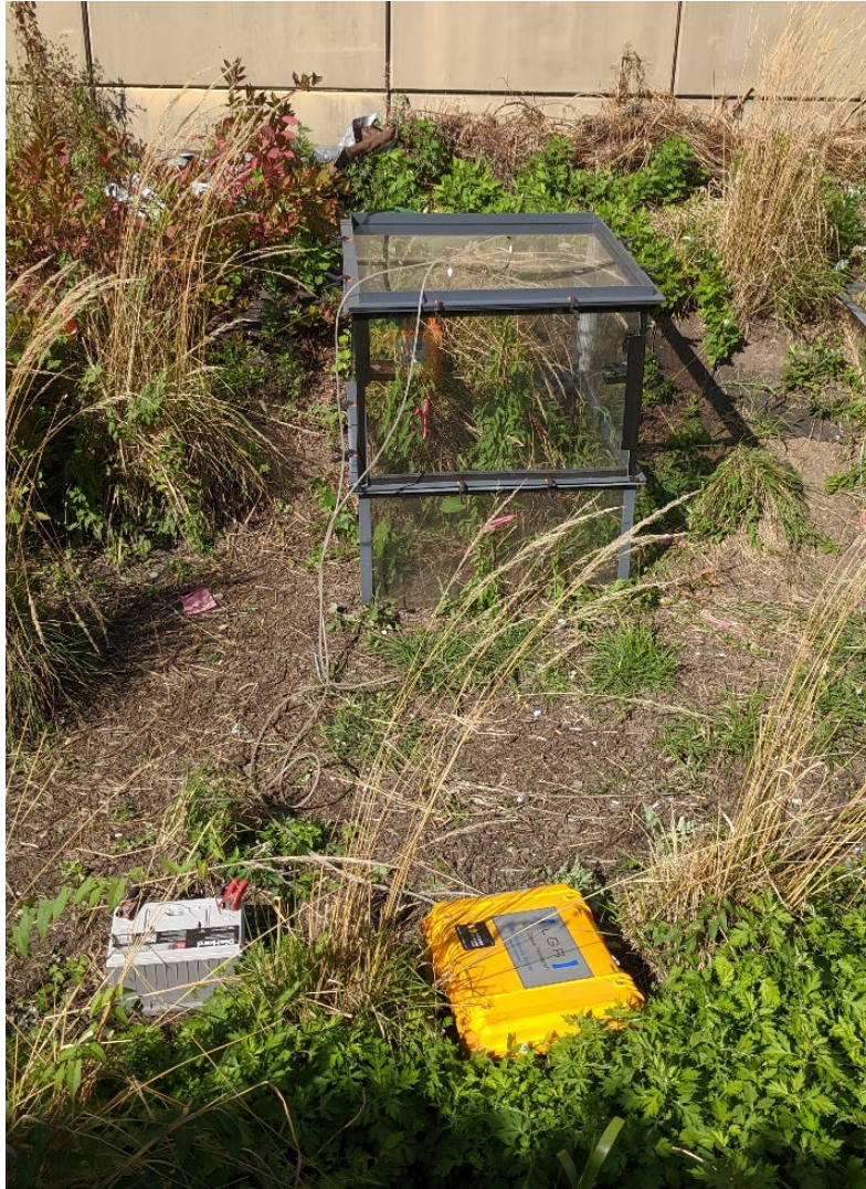
Figure S1. Setup used for chamber flux measurements, with the larger collar ( 92 \times 92 cm upper surface) and chamber ( 92 \times 92 \times 62.5 cm) shown. The gas analyzer (yellow) and its battery (grey) are in the foreground.
