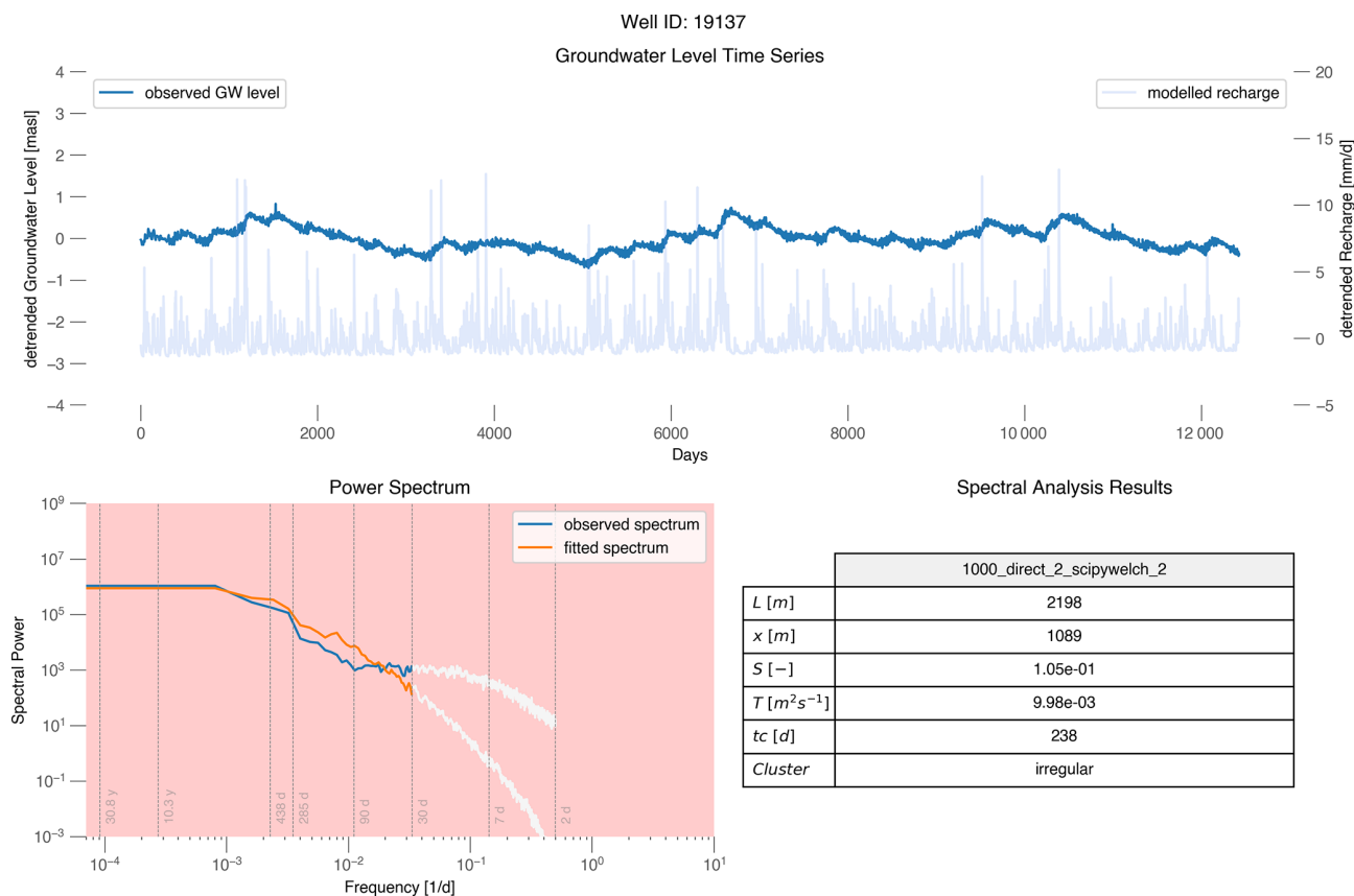
Figure A8. An example of a summary of analysis for a groundwater well of the category irregular . The figure shows the observed groundwater level time series and the modeled mHM recharge (Marx et al., 2021), the resulting power spectra for the observed groundwater level and the fitted spectrum with the semi-analytical solution. Only the colored part of the spectrum up to a frequency corresponding to 30 d was taken for the goodness of fit evaluation. The table summarizes the results of the workflow for the selected parameter set. In the presented time series and spectrum, multiple dominant frequencies can be observed: Long-term and multi-annual fluctuations with periods of decades, seasonal fluctuations with a period of a year and short-term fluctuations with periods of weeks to even days. The latter can be most likely attributed to barometric pressure changes in the atmosphere, as variations in summer are less than in winter times. The diverse set of present frequencies in the signal result in a complex shape of the spectrum with several breakpoints. Our simplified semi-analytical approach with a recharge product taken from a land surface model fails to capture the complexity of the processes of this groundwater level fluctuation and was consequently categorized as irregular.
