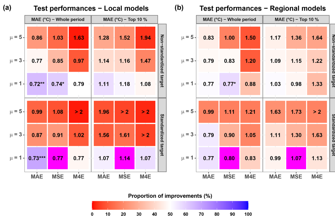
Figure 2. Median test performances (MAE, in °C) of the local models (a) and the regional models (b) according to the loss function used for training. These median values were computed from a set of 21 \times 4 = 84 points for the local models and 21 \times 7 = 147 points for the regional models. Note that the models we kept for test do not necessarily share the same lookback. Colours indicate the proportion of cases for which the use of the loss function yielded better results than the reference loss function (MSE with standardization, shown in magenta). Asterisks indicate that the custom loss function is significantly better than the reference loss function according to the one-sided binomial test: * for a significance threshold of 5 %, ** for a threshold of 1 %, and *** for a threshold of 0.1 %.
