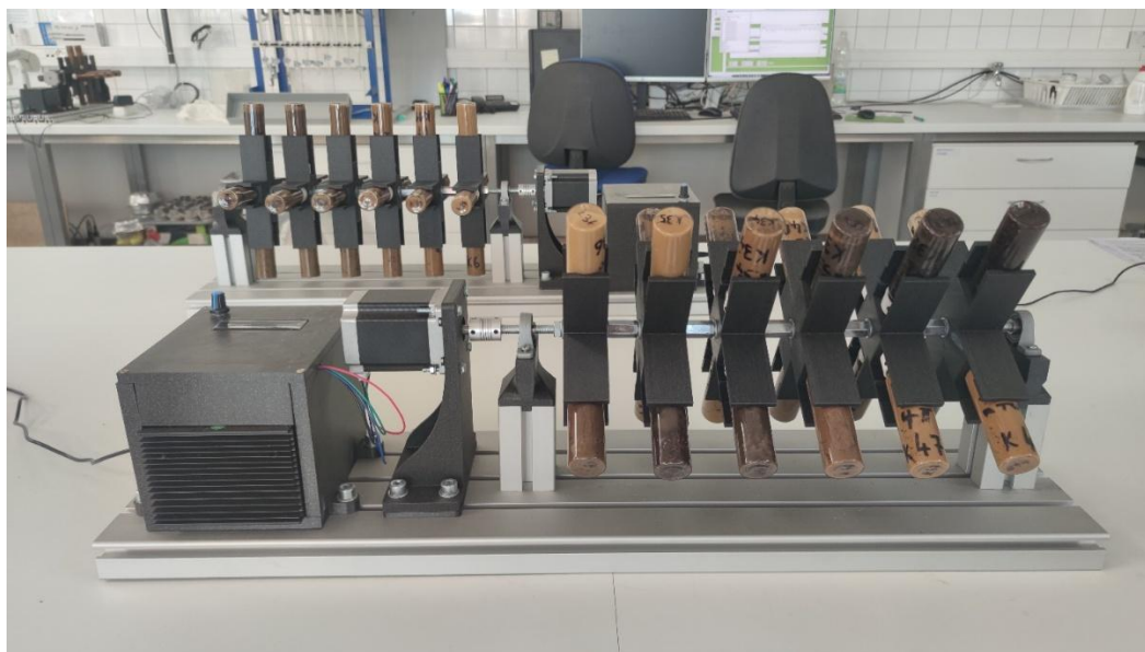
Figure S2. Custom-built laboratory apparatus designed to ensure homogeneous mixing of soil and added water through controlled mechanical motion of sealed sample vials prior to analysis.
