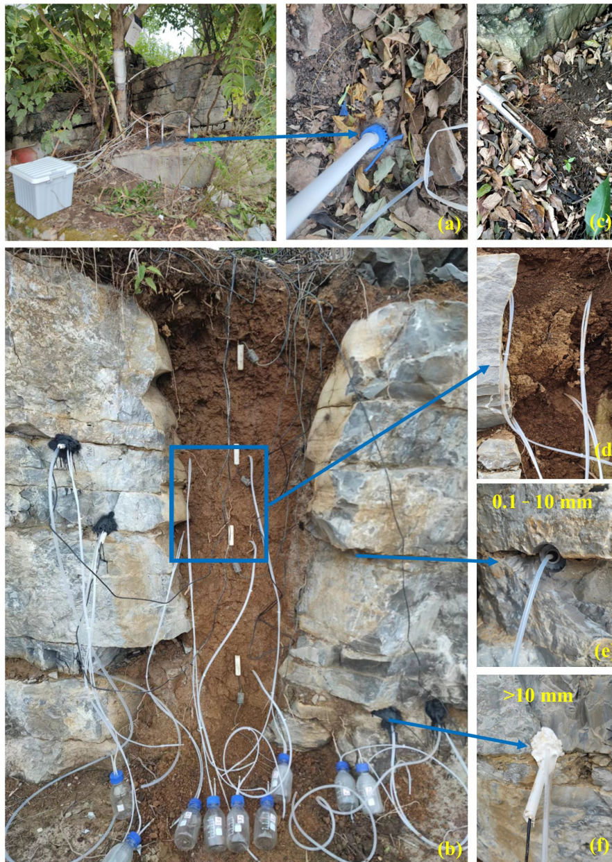
Figure A1. Field photographs illustrating soil and rock water sampling procedures. (a) Vertical boreholes drilled at sites C, D, and E with water sampling devices installed at predefined depths. (b) Horizontal boreholes drilled into exposed bedrock outcrops at sites A and B with sampling devices installed within the soil–rock profile. (c) Collection of soil samples for laboratory extraction of bulk soil water. (d) Collection of mobile soil water using suction lysimeters installed in soil layers. (e) Collection of rock fracture water from narrow fractures (aperture approximately 0.1–10 mm) with little or no soil infill. (f) Collection of infilled rock fracture water from wider fractures (> 10 mm aperture) largely filled with soil or fine sediments.
