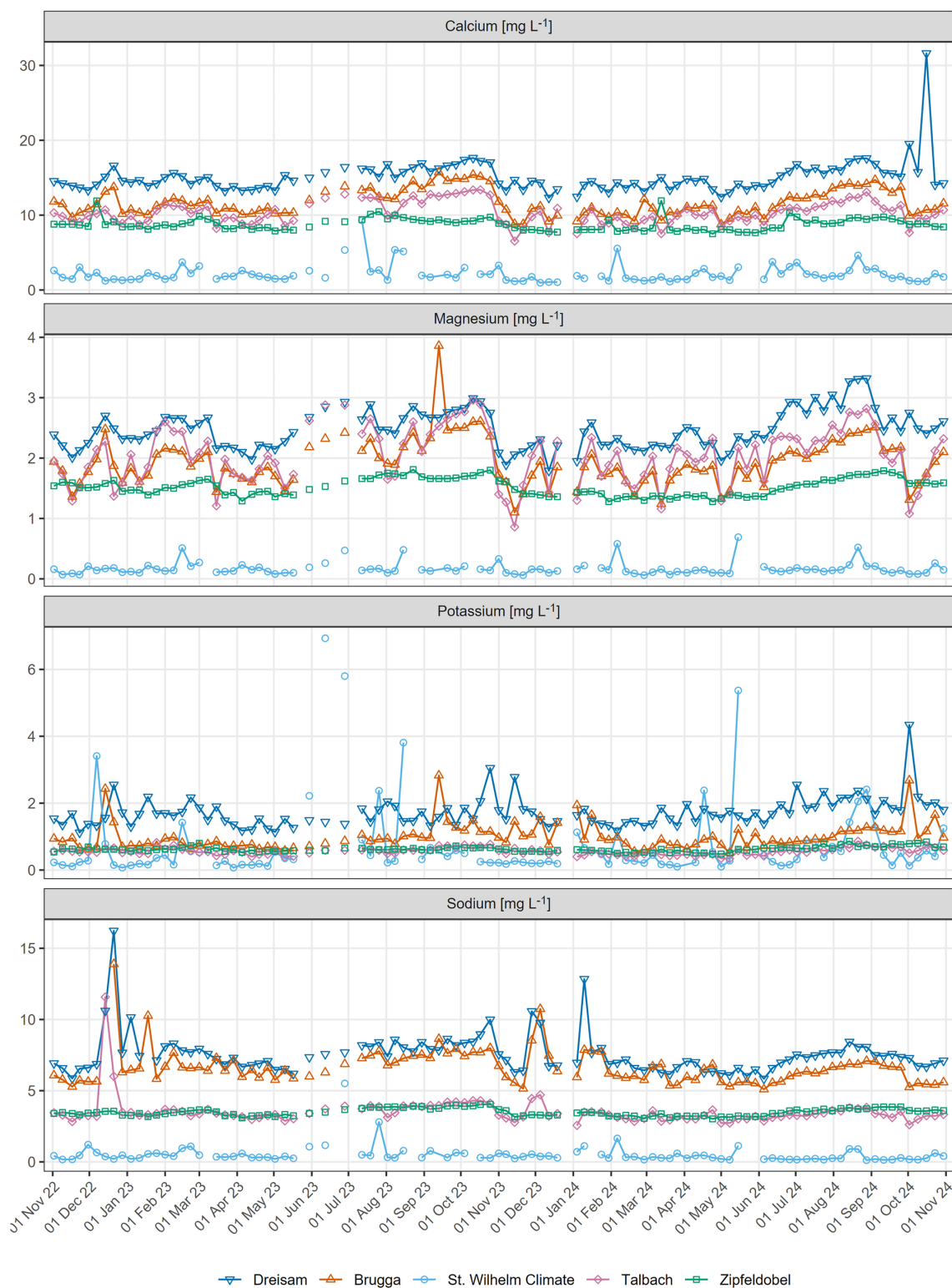
Figure F3. Time series of cation tracer data recorded in surface waters and precipitation for the hydrological years 2023 and 2024.
