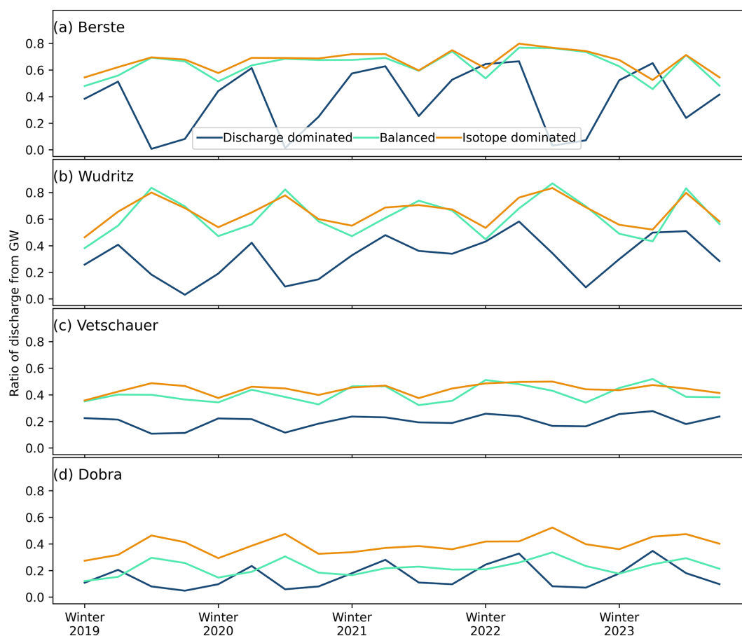
Figure 6. The mean ratio of seasonal runoff from groundwater storage at each catchment (winter, spring, summer, fall of each year along the x axis). The results were calculated from the discharge dominated, balanced and isotope dominated solutions in schemes 2–5.
