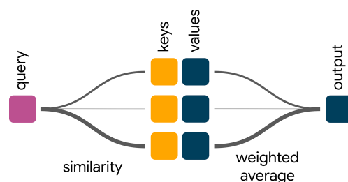
Figure D1. High-level illustration of attention. The query vector (left) is compared to each key vector (middle), and the corresponding value vectors are merged in a weighted average according to the similarity measure, producing the attention output (right).
