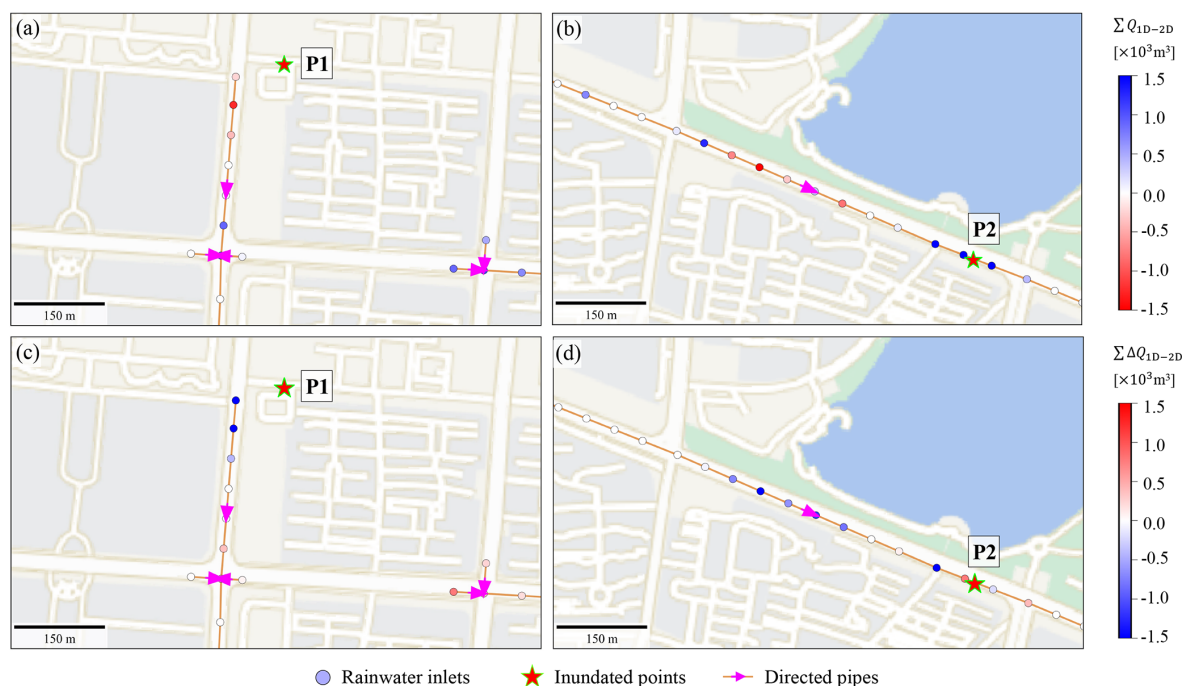
Figure 11. Comparison of accumulated discharges at rainwater inlets during the July 2022 storm. (a–b) RSN simulated discharges. (c–d) Simulated discharge differences between RSN and FSN defined by RSN minus FSN. Basemaps are provided by Tianditu ( https://map.tianditu.gov.cn/ ).
