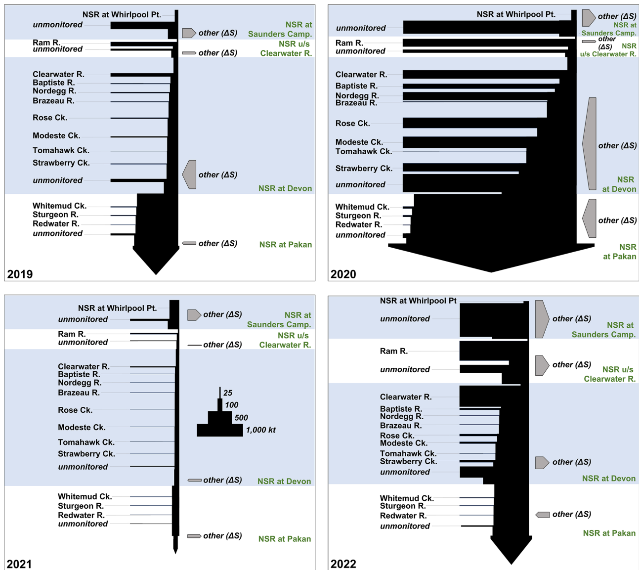
Figure 5. Total suspended sediment (TSS) export arrow diagrams of the North Saskatchewan River (NSR) basin for the water years (November to October) of 2019 to 2022. Tributary and storage exchanges are represented by horizontal arrows and NSR mainstem stations and reaches are shown as vertical arrows. Alternating shading delineates NSR mainstem reaches. Relative station spatial separations not to scale. Medians of all export models were used to construct mass arrows.
