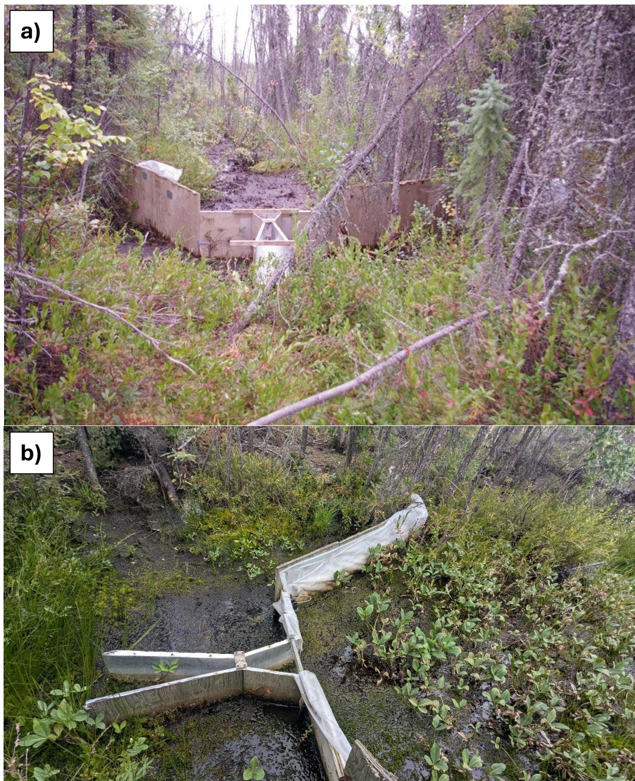
Figures S1: Cutthroat flume installed at the West sub-basin outlet West1 in a) 2014 (i.e., before the late-season wildfire in October 2022), and b) 2024 (i.e., after the late-season wildfire in October 2022).
