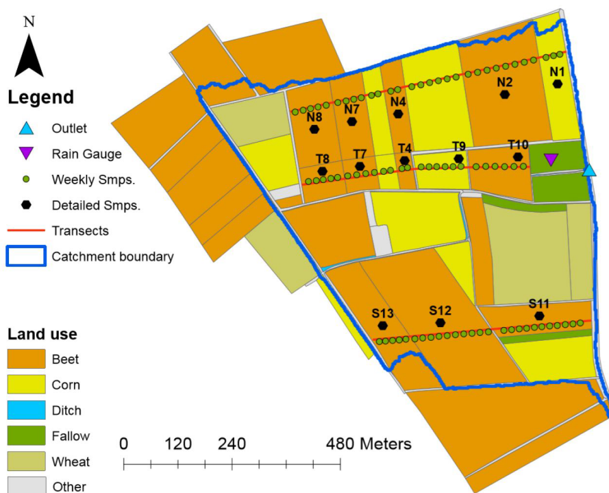
Figure 1. The Alteckendorf headwater catchment (Bas-Rhin, France) showing the experimental setup, including three transects, i.e. north, valley, and south (weighted samples collected at green dots along the red lines), and plot sampling (black dots). Land use for 2016 is also displayed. The “other” category includes roads, grass strips, and orchards.
