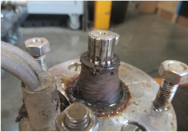
Figure S2: State of the submersible pump after running for five months during the high flow, winter period at the Naizin catchment. 10 Deposition of primarily organic material within the hydraulic parts of the pump and strong wear of the mechanics can be seen.
