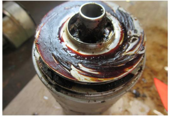
Figure S2: State of the submersible pump after running for five months during the high flow, winter period at the Naizin catchment. 10 Deposition of primarily organic material within the hydraulic parts of the pump and strong wear of the mechanics can be seen.
