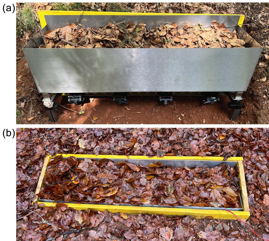
**Figure 2.** (a) Lysimeter container on the frame. (b) Fully installed FFGL aligned with the location.
