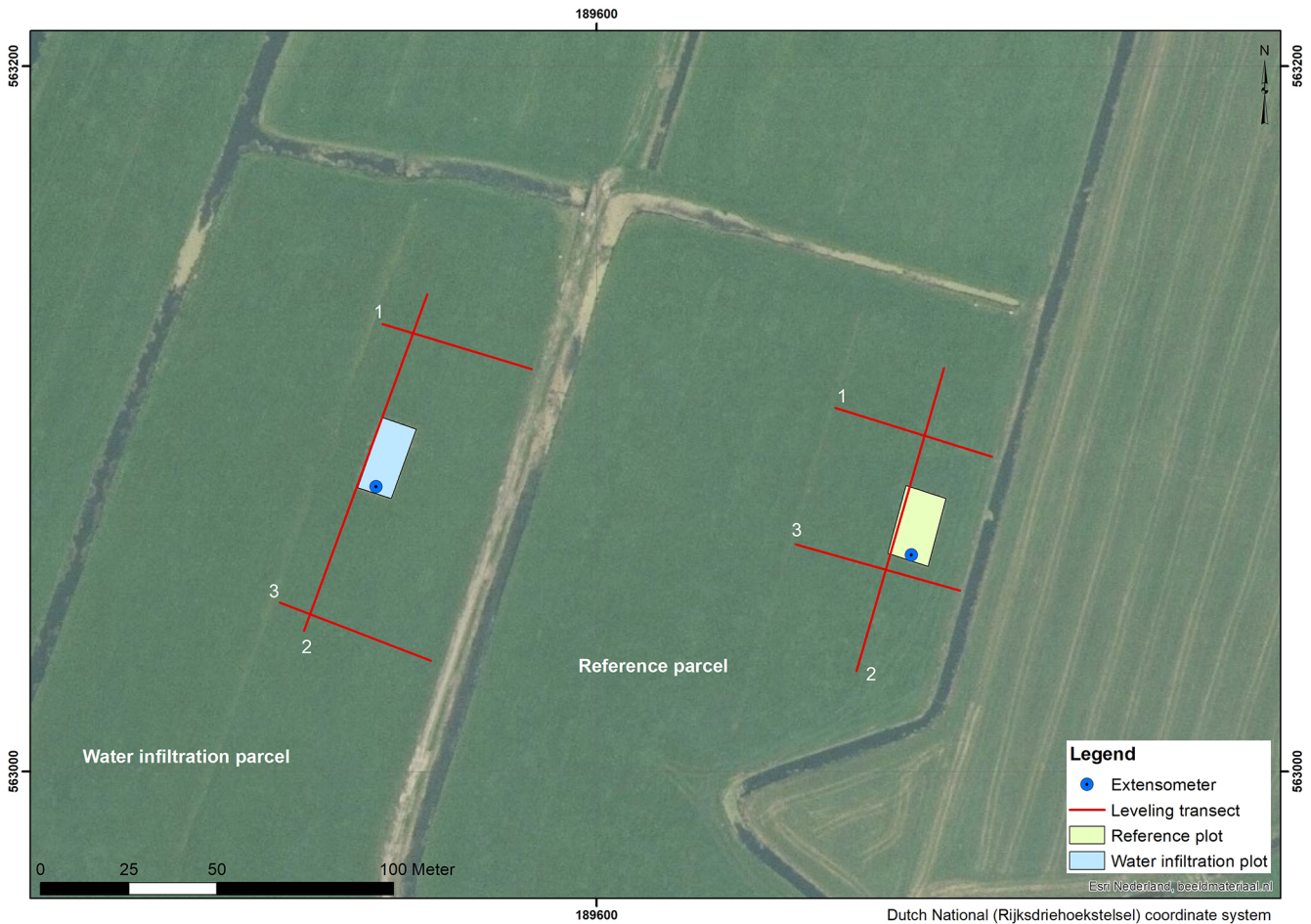
Figure 4. Position of field plots, spirit leveling transects, and extensometers in the reference and PWIS parcel at Aldeboarn.
