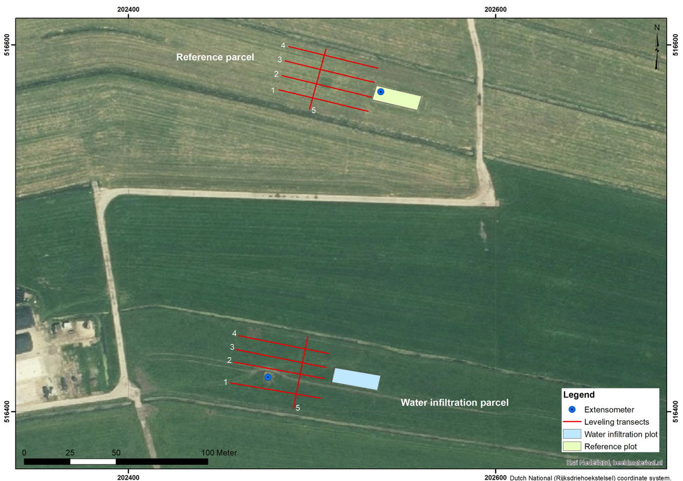
Figure 5. Position of field plots, spirit leveling transects, and extensometers in the reference and PWIS parcel at Rouveen.
