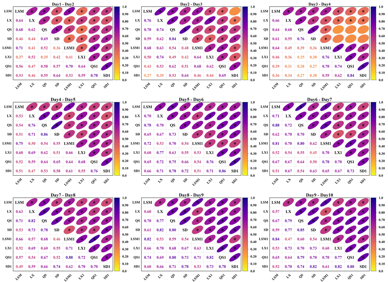
Figure 10. Partial results of the correlation analysis for daily runoff at multiple sites (LSM, LX, QS, and SD represent the runoff sequences of the current day, while LSM1, LX1, QS1, and SD1 represent the runoff sequences of the previous day).
