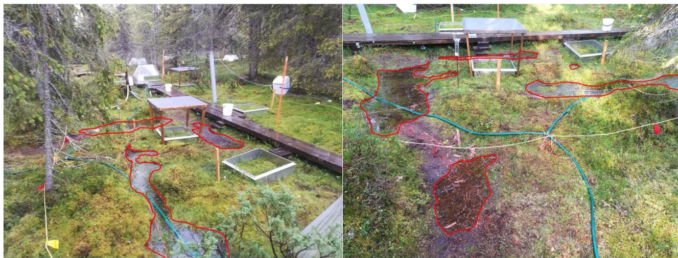
Figure S4. Surface ponding in the EP during irrigation.
