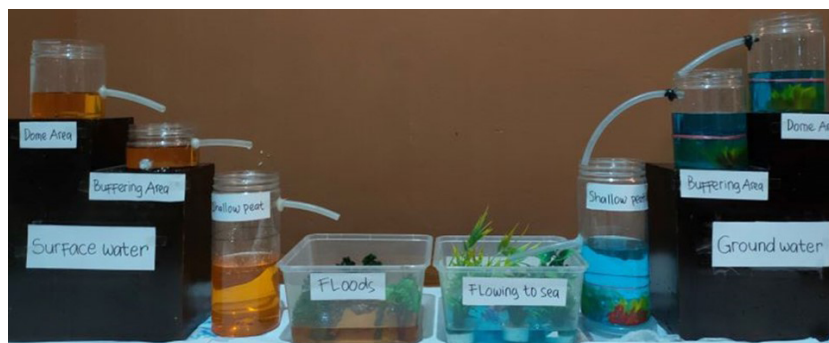
Figure D3. Simple water balance model of the H 2 Ours game in the Pawan–Kepulu peatland to show the dynamics of changes in hydrological conditions as a result of the changes in land use and canal density. The red line in each tank in the groundwater system represents the fire vulnerability threshold.
