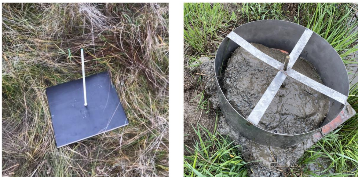
Fig. S10. Photographs of sedimentation plates. Sedimentation plate deployed on floodplain surface (left). Sediment yield after retrieving sedimentation plate placed in channel, using a cylindrical frame to prevent sediment losses to water (right).
