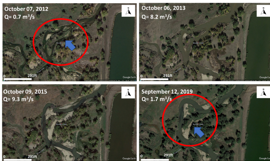
Figure 1. Change in channel width in Boulder Creek, Colorado, before (2012) and after (2013–2015–2019) a flash flood in 2013 (© Google Earth imagery). The discharge reported here is the daily discharge measured at USGS 06730200 Boulder Creek at North 75th St. near Boulder, Colorado. The red circles denote the section of the channel that has changed over the years, and the blue arrows show the missing channel from the years 2012 to 2019.
