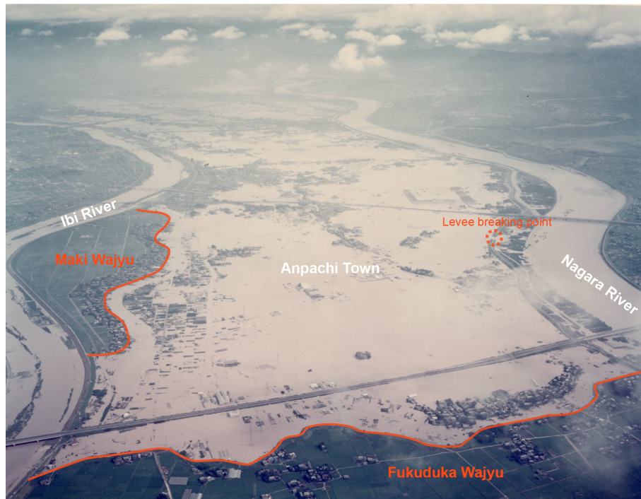
Figure 5. September 1976 flooding. The orange lines in the photo indicate remaining ring levees. The Nagara River levee broke, and the floodwaters flowed out onto the floodplain where Anpachi was located. However, the floodwaters were prevented from expanding into the inundated area by the remaining ring levees (this image is courtesy of the Ministry of Land, Infrastructure, Transport and Tourism).
