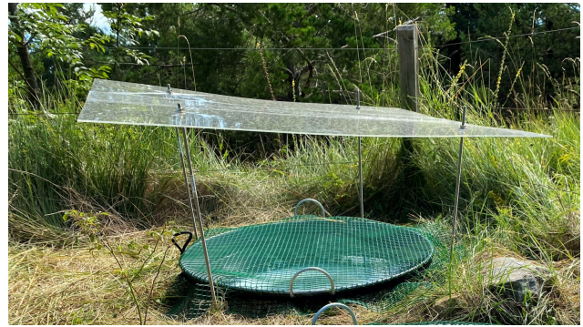
Figure 1. View of the steel experimental pan. The pan was partly buried in the ground and protected against precipitation by a lid of clear methacrylate installed 0.5 m above the pan's surface, to allow air circulation, and against large animals drinking by a net.
