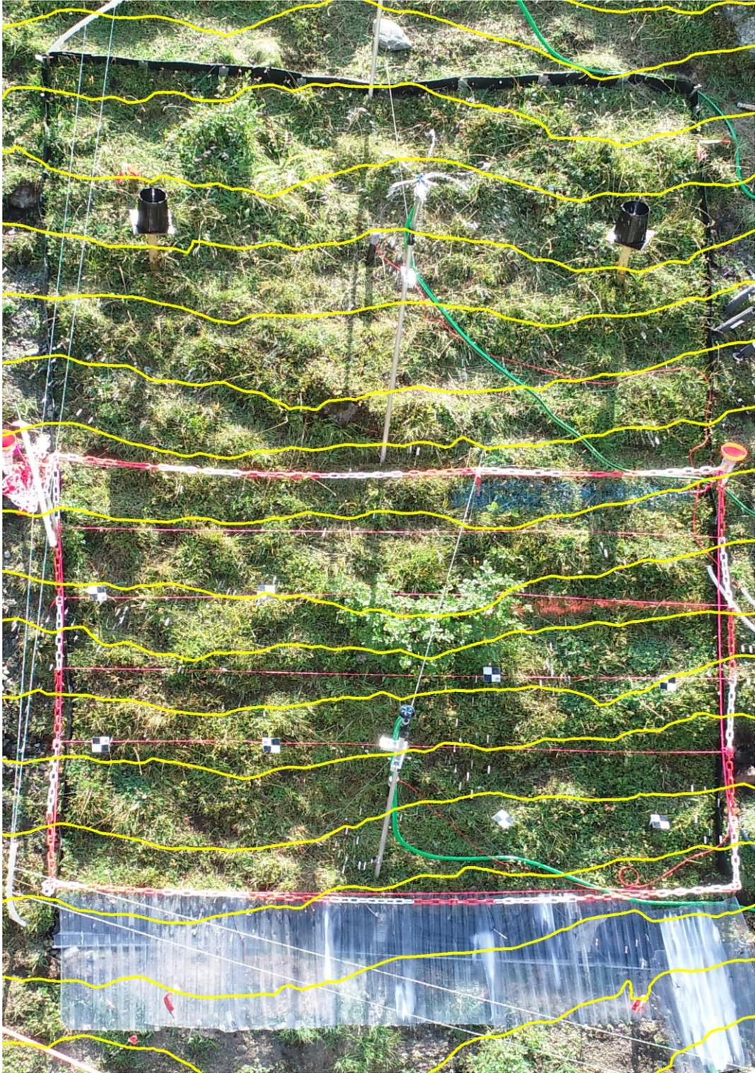
Figure S2: Georeferenced daylight drone photo of the 1860M plot with the 50 cm contour lines (yellow lines).
