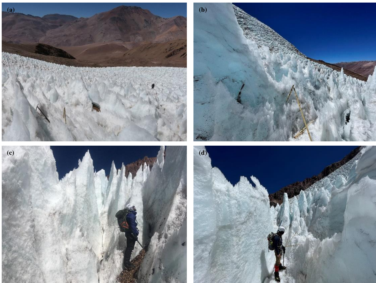
Figure S3: Images of ablation stakes and penitentes on Tapado Glacier. (a) Ablation stake in summer 2020, (b) Ablation stake in summer 2021, (c) and (d) 3-4 m penitentes in summer 2021.
