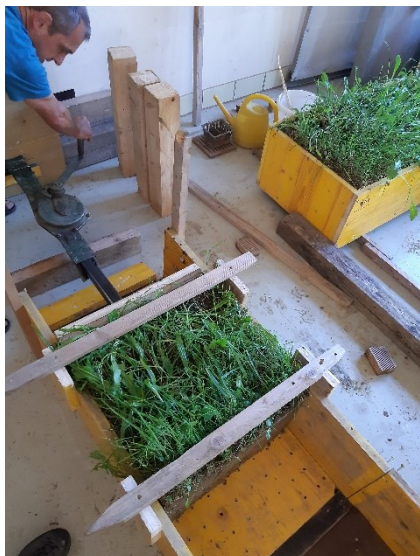
Pushing the two soil blocks together using a rack and pinion jack
