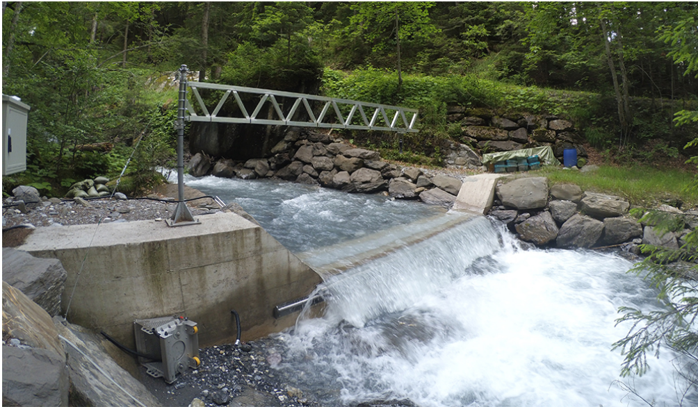
Figure S3: River stage measure at the outlet. The streamflow is here measured between 0.96 and 1.13 \text{ m}^3 \cdot \text{s}^{-1} .
