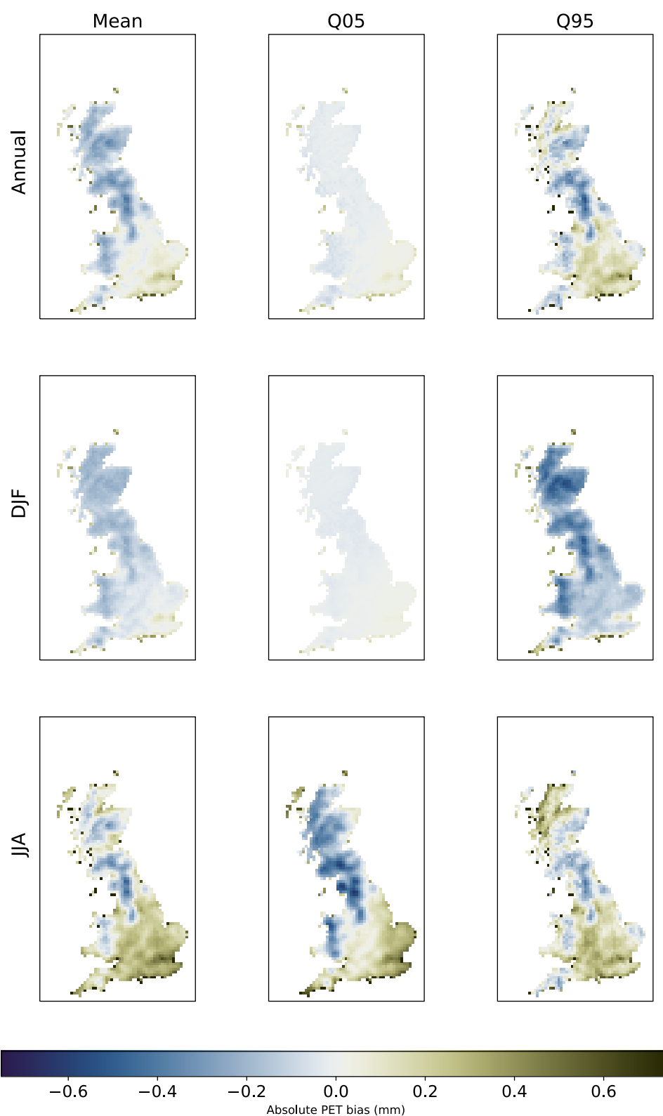
Figure S2. Mean PET biases (mm) in UKCP18-RCM for 1981-2010. The bias for each ensemble member was computed and the mean across the ensemble is shown here. Q05 and Q95 are the biases in the 0.05 and 0.95 quantiles respectively.
