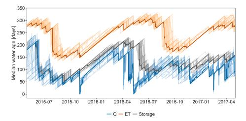
**Figure 6.** Median water age in stream runoff (Q, blue), the catchment storage (S, gray), and the evapotranspiration flux (ET, orange). Age estimates shown for the best simulation (dark color) and the top 100 simulations (light color).
