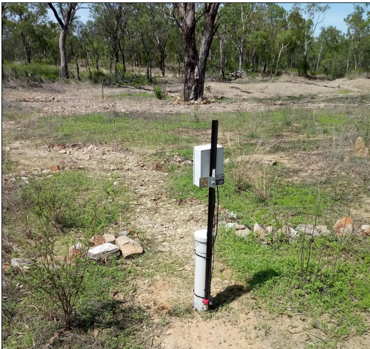
Figure S2 PASS sampler located in catchment drainage channel, upstream of the remediated gully.
