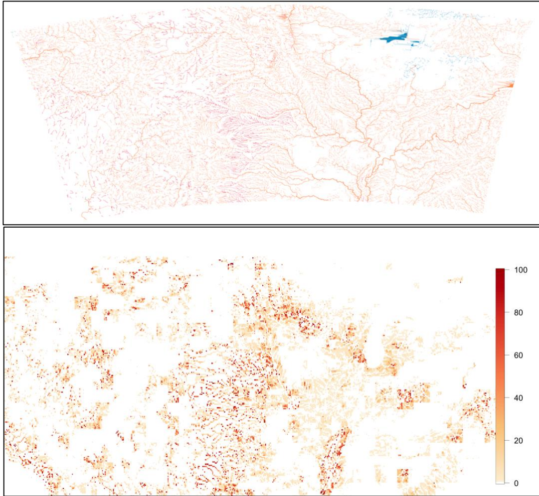
Supplementary Figure S13. Comparison of streamflow depletion (% change in discharge) since predevelopment (1900-2008) as simulated with ParFlow-CLM by Condon and Maxwell (2019) with the estimates with the analytical framework (assuming q > q_{crit} , t > t_{crit} or q < q_{crit} , t \gg t_{ef} ); top: results from Condon and Maxwell (2019); bottom: estimates from the analytical framework; note that the Condon and Maxwell results represent cumulative dQ as fraction of Q , whereas the results from the analytical framework represent marginal dQ as a fraction of Q ; this makes the results only comparable for the headwaters.
