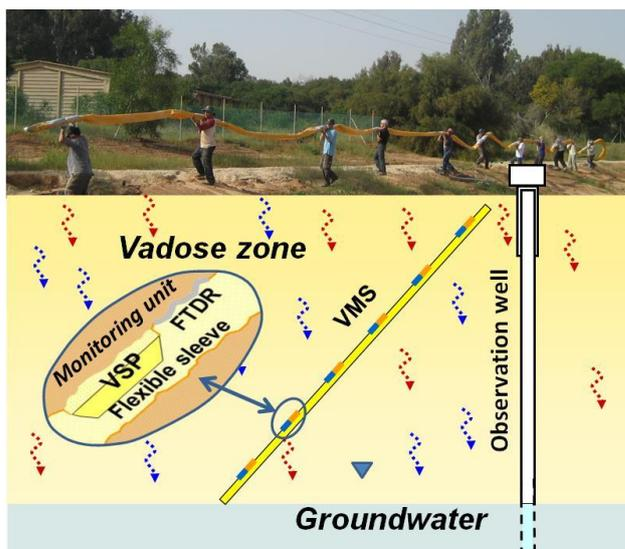
Figure S1 - The Vadose Zone Monitoring System as it is carried prior to its installation (top), and a general layout of the VMS systems when placed in the soil (bottom).
