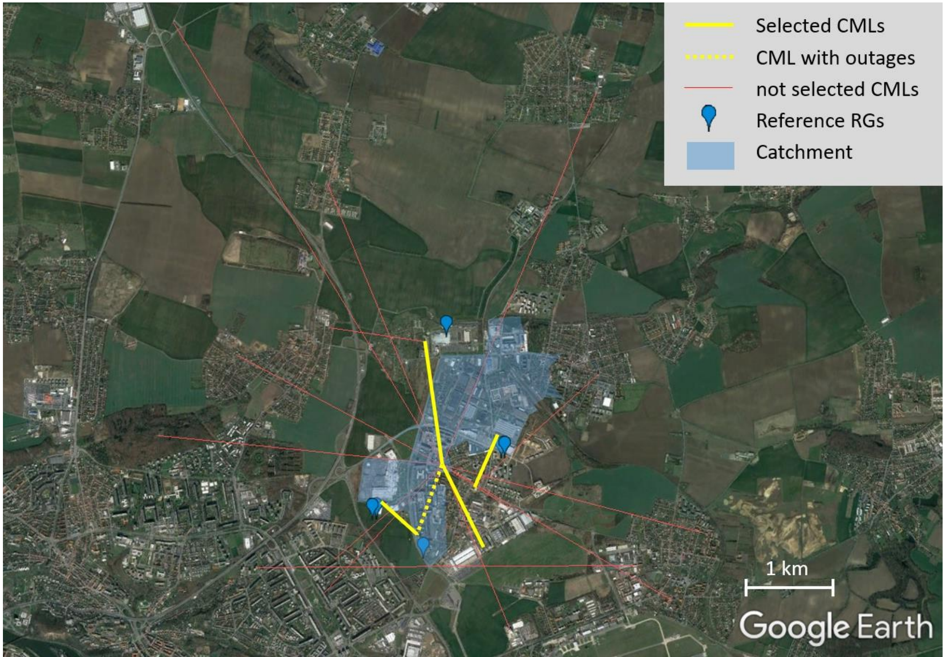
Detailed view on the network of commercial microwave links (CMLs) operated by T-Mobile (CZ) in the catchment Prague-Letnany together with reference rain gauges (RGs) operated for experimental purposes. Exact coordinates of CMLs are not provided due to confidential character of this information.
