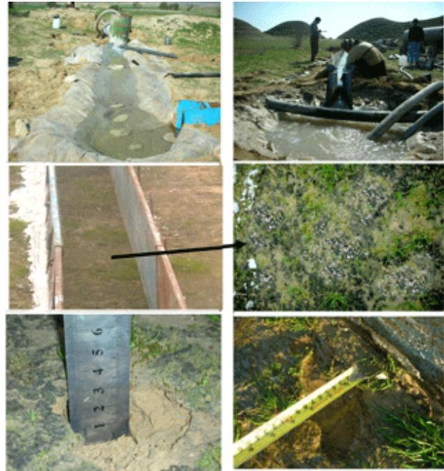
**Figure 1.** Flume, water supply, retention pond, overflow pipe, and Parshall flume (top photos); flume surface and vegetation (grass and pale pink lichen patch) in the rangeland (middle photos); sample of initiated head cut with height of 3 cm in rangeland (bottom left photo); and abandoned land (bottom right photo).
