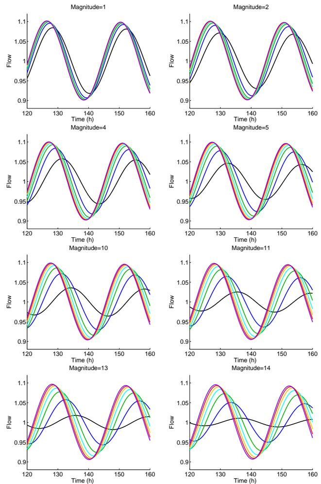
**Figure 7.** Flows at the outlet of each magnitude link using different  $k$  in each river simulation. The  $k$  values (with units of  $\text{h}^{-1}$ ) are 0.38, 0.7, 1.02, 1.34, 1.66, 1.98, and 2.30 and are colored black, blue, green, cyan, orange, red, and purple, respectively. The flows are normalized about the average flow.
