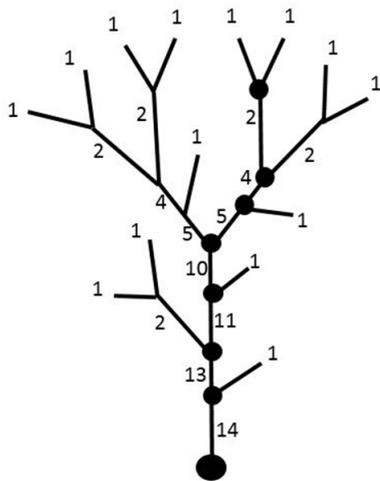
**Figure 5.** The Mandelbrot–Vicsek tree of magnitude 14. The magnitude of each link is written next to the link. One link of each magnitude is distinguished by the dots along the network.
