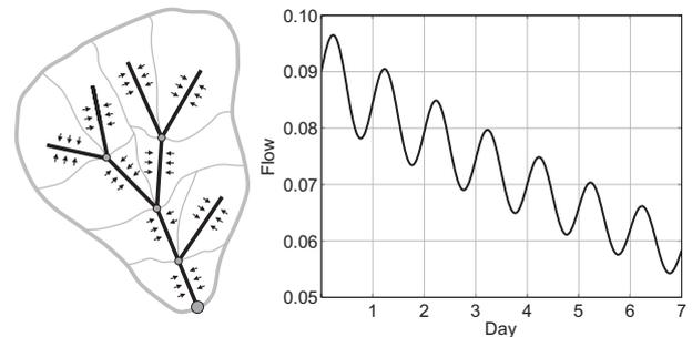
**Figure 2.** The left panel shows how runoff enters the river network as lateral flow from each hillslope to its adjacent link. The right panel shows a sample baseflow pattern given by Eq. (1) using  $A = 0.003 \text{ [h}^{-1}\text{]}$ ,  $B = 0.08 \text{ [L s}^{-1}\text{]}$ ,  $C = 0.008 \text{ [L s}^{-1}\text{]}$ ,  $\nu = \frac{1}{24} \text{ [h}^{-1}\text{]}$ , and  $\phi = 0 \text{ [h]}$ .
