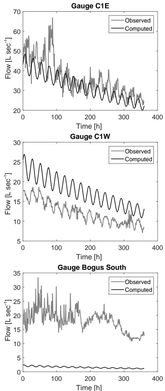
**Figure B1.** Observed streamflow and streamflow fitted using Eq. (16) at three upstream gauges in the Dry Creek Experimental Watershed: Con1East (top), Con1West (center), and Bogus South (bottom).
