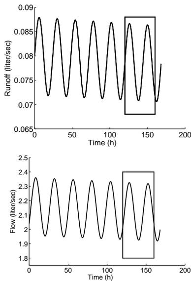
**Figure 6.** Sample runoff pattern (top) and resulting streamflow solution at the outlet in the uniform case (bottom) for  $k = \frac{v}{L}$ . To examine the oscillations more closely for different velocities, we will focus on a small section of the solution (highlighted by a box in each panel).
