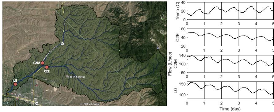
**Figure 1.** The left panel shows the Dry Creek watershed in Idaho. The right panel shows temperature (top), streamflow at gauge C2E near the center of the watershed (second), streamflow at gauge C2M (third), and streamflow at the outlet of the watershed (bottom). To demonstrate the delay in phases, a vertical line at the beginning of each day is included in each graph.
