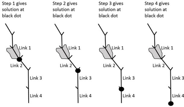
**Figure 3.** To determine the solution at any point, we consider runoff on only one hillslope (adjacent to link 1 in this case), and we trace the effects of that runoff downstream with no additional runoff from any subsequent hillslopes.
