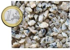
Here you can see gravel as it is below the surface. Geologists say that fine grained gravel has also small pore spaces. Do you know what is meant by the term pore space?
