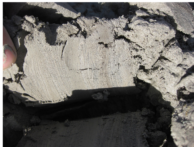
Figure 8. Fine sand sample with thin silty intercalations – test field FS/SU1 (Ravnik).
