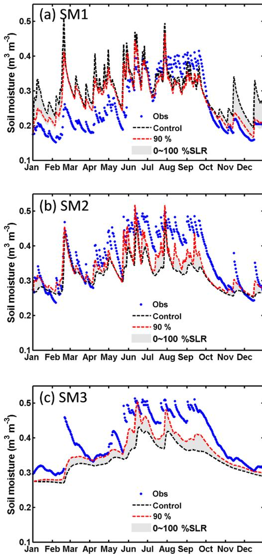
**Figure 5.** Simulated and observed soil moisture for the LHC site at depths of (a) SM1 (0–20 cm), (b) SM2 (20–70 cm) and (c) SM3 (70–170 cm). Observed results are shown as blue dots. Simulations with SLR = 0 (i.e., control run, without stem–root flow) and SLR = 90 % are shown as black dashed and red dashed curves, respectively. The area of grey shading enclosed by SLR = 0 % and 100 % indicates the possible range of the stem–root flow effects. All simulation results are daily averages.
