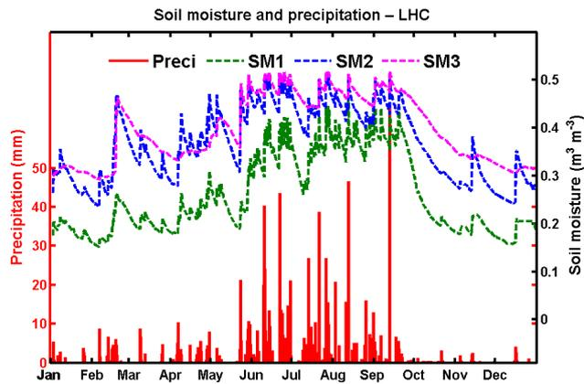
**Figure 2.** The hourly soil moisture (curves, right axis) and precipitation (red bars, left axis) observed at LHC during 2010. SM1, SM2 and SM3 represent soil moisture at 10 cm (green dashed curve), 40 cm (blue dashed curve; average of 30 and 50 cm observations) and 90 cm (magenta dashed curve), respectively.
