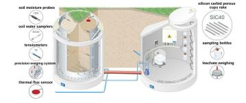
**Figure 1.** Schematic drawing of a lysimeter (left) as used in SoilCan attached to the central service pit (right).
