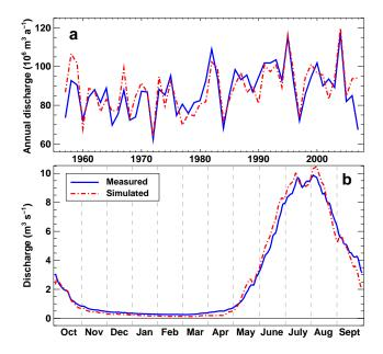
**Fig. 4.** Validation of discharge from the Rhonegletscher catchment calculated using GERM to measurements at Gletsch. (a) Annual runoff volume, and (b) stacked daily runoff hydrographs for the period 1957–2006.
