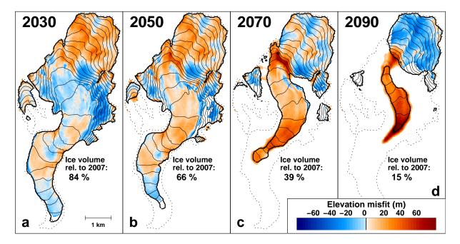
Fig. 7. Comparison of surface elevation and glacier extent calculated for Scenario 2 (median) using the ice flow model (M) and the  $\Delta h$ parameterization (P) for Rhonegletscher. Coloured areas indicate ice coverage as calculated by the ice flow model. The colours refer
