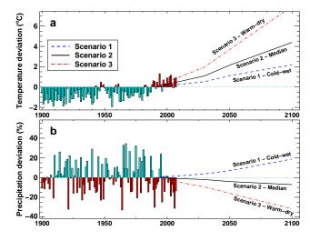
**Fig. 6.** Deviations of annual (**a**) mean air temperature and (**b**) precipitation sums from the the period 1980–2000. Measured data for the 20th century are displayed by bars, annual trends as assumed by Scenarios 1–3 (Table 1) are shown until 2100.
