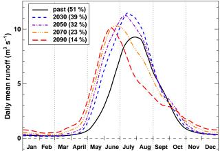
**Fig. 13.** Projected change in the hydrological regime of the Rhonegletscher catchment according to Scenario 2 (median). Measured discharge in the past refers to the 1961–1990 average. Numbers in brackets indicate the glacierization of the drainage basin.
