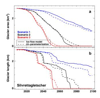
**Fig. 11.** Calculated (a) glacier area and (b) length based on the ice flow model and the  $\Delta h$ -parameterization according to the three climate scenarios (Silvrettagletscher).
