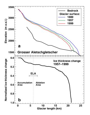
**Fig. 1. (a)** Observed long-term surface elevation changes in a longitudinal glacier profile for a large alpine valley glacier (Grosser Aletschgletscher). **(b)** Distribution of ice thickness change along the glacier in 1957–1999. Changes in ice thickness are small in the accumulation area and largest near the glacier terminus. The variability in the equilibrium line altitude (ELA) over the 20th century is shown.
