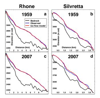
**Fig. 5.** Validation of the coupled ice flow and surface mass balance model over the 20th century using field data. Comparison of observed and calculated glacier surface on a longitudinal profile in 1959 and 2007. Model runs were initialized in 1874 (Rhone) and in 1938 (Silvretta).
