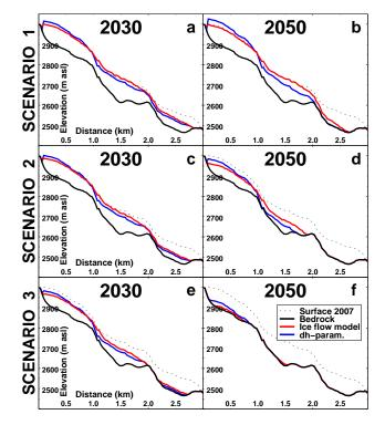
Fig. 10. Evolution of glacier surface elevation along a longitudinal profile calculated for Silvrettagletscher using the ice flow model and the  $\Delta h$ -parameterization. Results for different climate change scenarios are shown.
