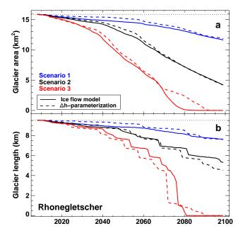
**Fig. 9.** Calculated (a) glacier area and (b) length based on the ice flow model and the  $\Delta h$ -parameterization according to the three climate scenarios (Rhonegletscher).
