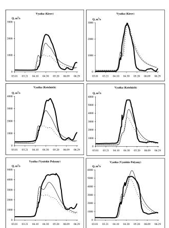
**Fig. 10.** Comparison of the observed hydrographs (bold line) with the hydrographs calculated from the constructed SWE fields (thin line) and from AE-DySno SWE maps (dashed line). (The left column presents hydrographs of the 2003 flood, the right column presents hydrographs of the 2005 flood).
