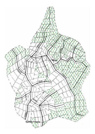
Fig. 8. Finite-element schematization of the Vyatka River basin (bold lines represent the channel network; thin lines represent the boundaries of finite elements; green labels mark the forested elements).
