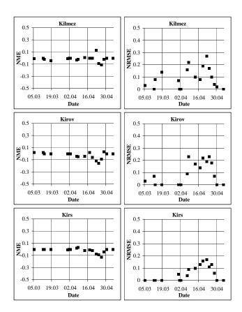
Fig. 5. Normalized mean error (NME) and normalized root mean square error (NRMSE) of simulated snow covered area in comparison with one obtained from NASA MOD10\_L2 maps for three Thissen polygons surrounding meteorological stations Kilmez, Kirov, and Kirs (forested pixels are not taken into account). 1 March 2002-30 April 2002.
