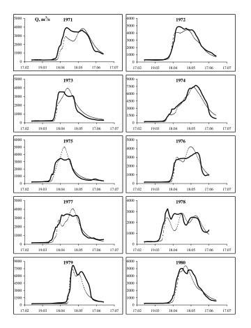
**Fig. 9.** Comparison of the observed (solid line) and calculated (dashed line) hydrographs at the gauge Vyatskie Polyany of the Vyatka River (the last ten years of validation period).
