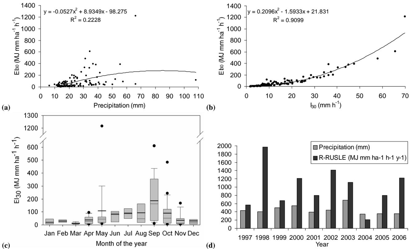
**Fig. 3.** Correlation between the runoff and rainfall erosivity values with their values of precipitation (a) and maximum intensity (b). Monthly values of runoff and rainfall erosivity in a box plot diagram (c). Annual values of precipitation and runoff and rainfall erosivity factor for the period 1997–2006 at the weather station of Canelles (d).
